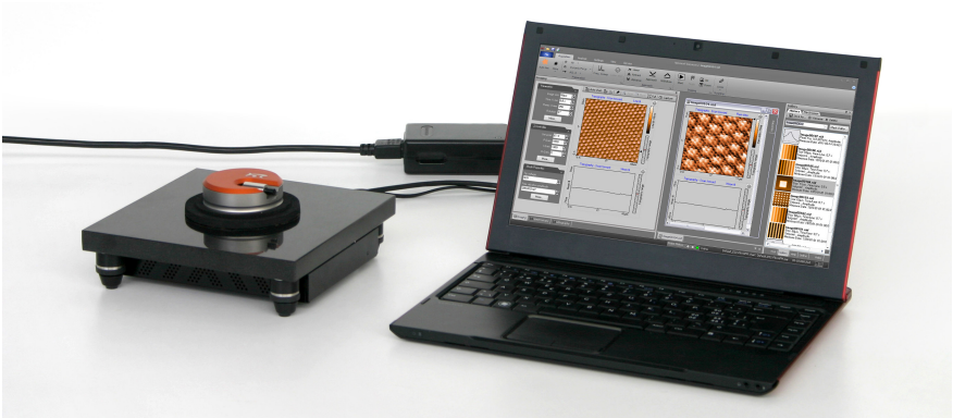
Figure 2-1: Measurement setup. Complete NaoSTM system with personal computer.
